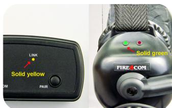
**9** Within a few seconds, the red and green lights will stop flashing and you will see a solid green light on the headset and a solid yellow Link light the base station, indicating the headset has been properly linked.
