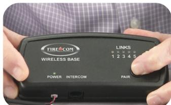
**7** To link the next headset, press and hold the Pairing button on the front of the base station until the remaining link lights begin to flash.
