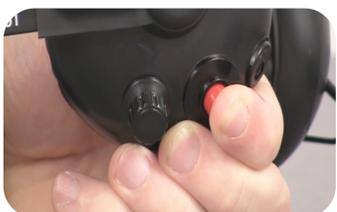
**8** Grasp the second headset you wish to pair and then depress and hold the push-to-talk button on the dome. Keeping the button firmly depressed, turn the headset on by twisting the volume control in a clockwise direction. The green light will flash initially when the unit is turned on, and then switch to flashing red and green lights. When this occurs, release the push-to-talk button.
